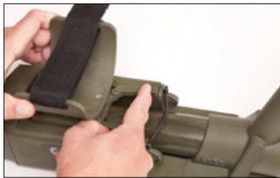
Armrest locking lever shown in open position.
