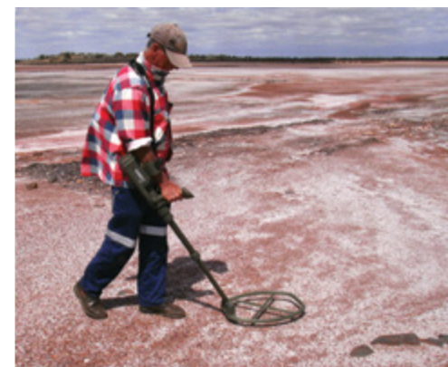
This moistened ancient salt bed, which also contains veins of iron mineralization, is an example of a non-uniform soil condition.
