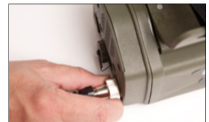
Hand-tighten connector collar.
