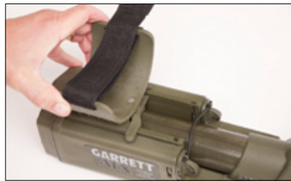
Armrest locking lever shown in locked position.
