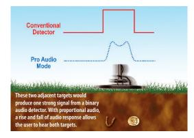
The AT Max International and AT Pro International each feature advanced. proportional (Pro) audio modes. This allows the user to: hear subtle changes in a target's response; better judge a target's size, shape and depth; and enjoy a much faster recovery time when detecting adjacent targets.
